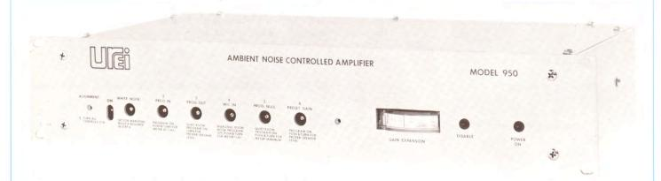
The UREI Model 950 "ANCA" is the first device to bring true precision to automatic P.A. level control. It compensates precisely for changes in background noise even while an announcement is in progress. The ANCA is inserted into the system immediately ahead of the power amplifier and takes full control of the announcement level.
